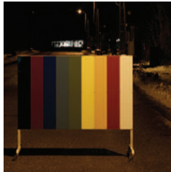
HST - High pressure sodium luminaire Poor colour rendering CRI < 35
